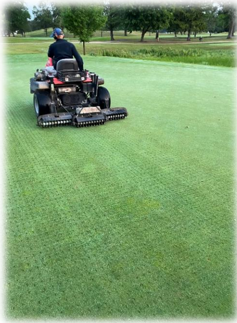
Taylor spiking greens, this breaks surface tension and allows gas exchange. Process is timed with greens topdressing and causes no disruption to play.
