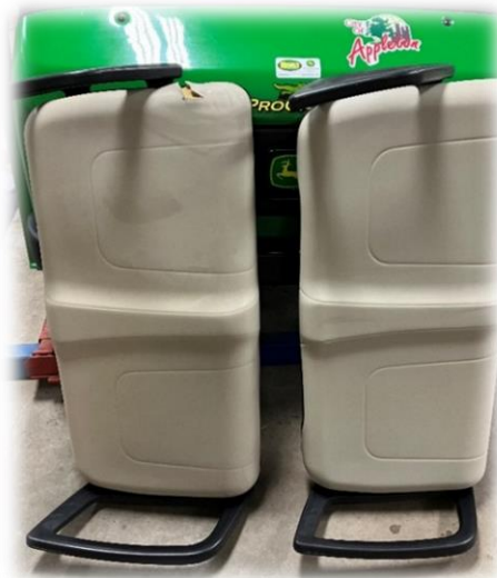
Old seat on left and new on right, top of left seat with tear. Damage consistent on the entire cart fleet.
