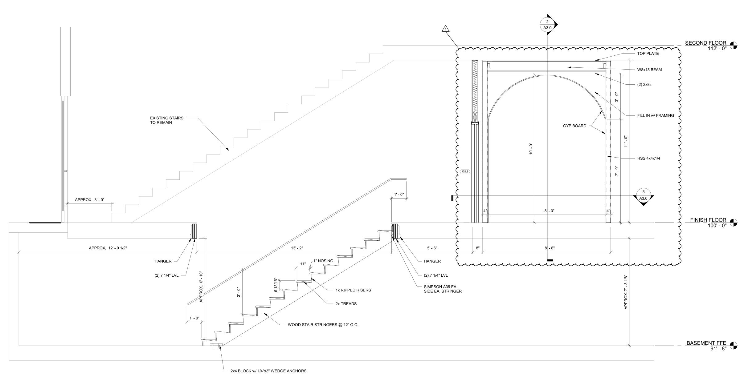
**STAIR SECTION** 1 /A3.0 SCALE = 1/2" = 1'-0"
