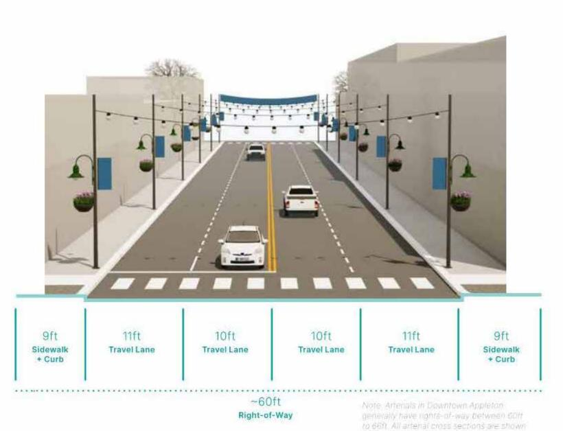
for a 60th-wide right-of-way to provide consistency. Rights of way wider than 600
