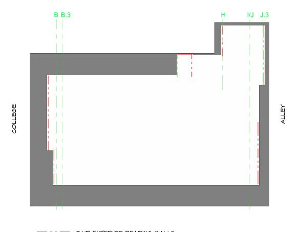
2 HR EXTERIOR BEARING WALLS X - - - 2 HR FIRE PROOFING OF PRIMARY EXISTING STRUCTURE (COLUMNS/BEAMS)
